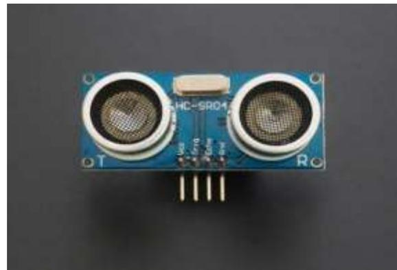
HC-SR-04 has an ultrasonic transmitter, receiver and control circuit.
