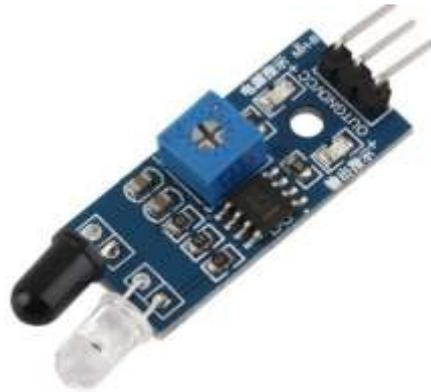
The emitter is simply an IR LED ([Light Emitting Diode](#)) and the detector is simply an IR photodiode. Photodiode is sensitive to IR light of the same wavelength which is emitted by the IR LED. When IR light falls on the photodiode, the resistances and the output voltages will change in proportion to the magnitude of the IR light received.
