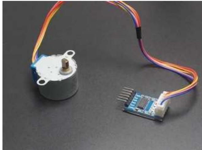
Step angle is the minimum angle that stepper motor will cover within one move/step. Number of steps required to complete one rotation depends upon step angle. Depending upon stepper motor configuration, step angle varies e.g.  $0.72^\circ$ ,  $3.8^\circ$ ,  $3.75^\circ$ ,  $7.5^\circ$ ,  $35^\circ$  etc.
