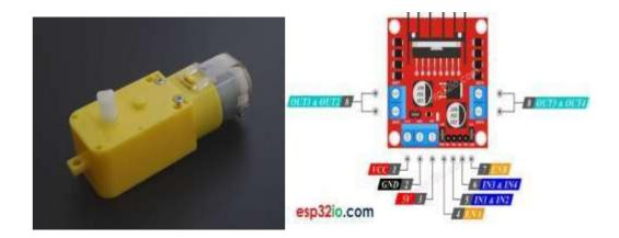
The working principle of DC motor is based on the fact that when a current carrying conductor is placed in a magnetic field, it experiences a mechanical force and starts rotating. Its direction of rotation depends upon Fleming's Left Hand Rule.DC motors are used in many applications like robot for movement control, toys, quadcopters, CD/DVD disk drive in PCs/Laptops etc.
