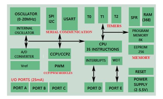
One of the main advantages is that it can be write-erase as many times as possible because it uses **FLASH memory technology**. It has a total number of 40 pins and there are 33 pins for input and output. PIC16F877A is used in many **pic microcontroller projects**. PIC16F877A also have much application in digital **electronics circuits**.
