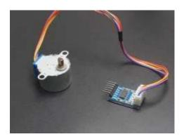
Step angle is the minimum angle that stepper motor will cover within one move/step. Number of steps required to complete one rotation depends upon step angle. Depending upon stepper motor configuration, step angle varies e.g. 0.72°, 3.8°, 3.75°, 7.5°, 35° etc.
