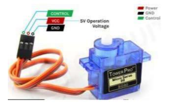
It is a closed loop system where it uses negative feedback to control motion and final position of the shaft. It is not used for continuous rotation like conventional AC/DC motors. It has rotation angle that varies from 0° to 380°.
